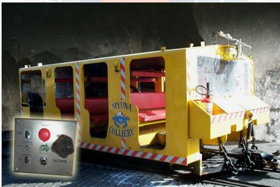
Tecom Australia has utilised STI Engineering radios for more than 8 years in their underground Shaft Management Systems (SMS). The SMS allows for reliable wireless control and voice communications from a trolley or skid to the winder.
